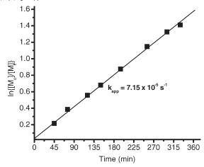
**Figure 1.**Semi logarithmic kinetic plots for the ATRP of MMA at 90 °C using different initiators. [MMA] = 4.68 M. [MMA]: [MBB]: [CuBr]: [BPIEP] = 100: 1: 1: 2.
