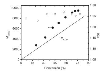
**Figure 2.** Dependence of molecular weight and polydispersity on conversion in the solution ATRP of MMA at 90  $^{\circ}$ C with [I] = 0.0468 M. Open symbols represent polydispersities and filled symbol represents  $M_n$ -(GPC).
